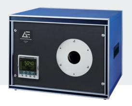
The Mikron® M305 blackbody calibration source uniquely combines portability with wide temperature range, high emissivity, and high accuracy. It is an ideal calibration unit where portability is required or where installation space is limited. Its spherical metal cavity design yields an emissivity of 0.995 over the temperature range of 100 to 1000°C (212 to 1832°F) with an aperture of 25 mm (1"). An integrally mounted PID controller adds to the unique versatility of this calibrator.
